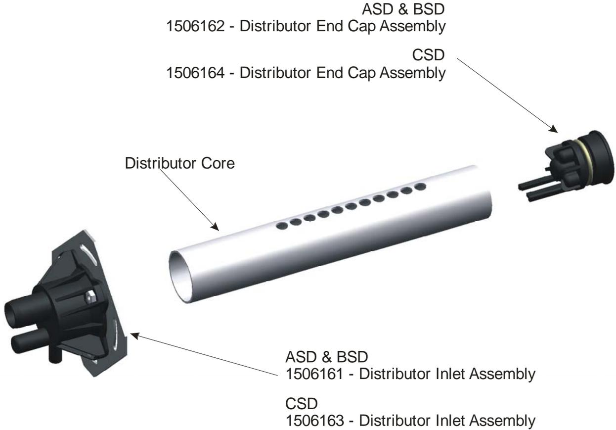
**Figure 46: Distributor Exploded View and Spare Parts**
