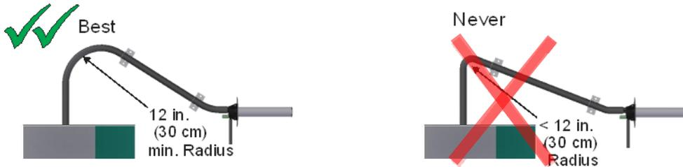
**5. Install traps on condensate lines at least 12" (30 cm) below connection.**
