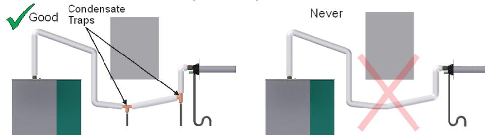
**8. Increase diameter either on down slope or install condensate trap.**
