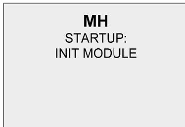
On the MHTC the LCD display will illuminate and the humidifier will perform a self-diagnostic sequence during which the LED's and internal components will be momentarily activated.
