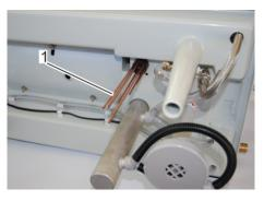
Fig. 26: Clean electrode rods
