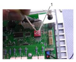
Fig. 21: Coding the humidifier
