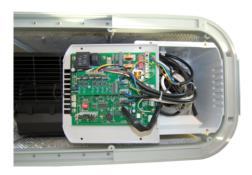
Fig. 72: Remove the control panel
