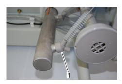
Fig. 67: Cleaning the stainless steel pipe
