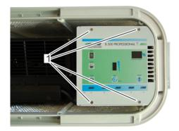
Fig. 19: Loosening the control panel
