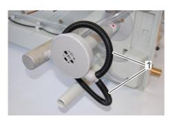
Fig. 50: Attach pump hoses
