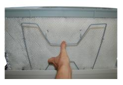
Fig. 28: Remove filter bracket
