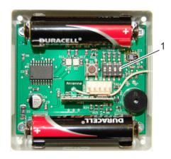
Fig. 17: Coding the wireless sensor system
