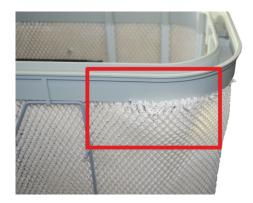
Fig. 10: Wrong fit of filter
