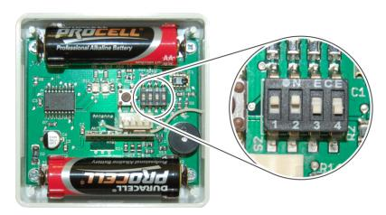
Fig. 15: Slide controls for coding
