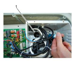
Fig. 73: Pulling out the UV lamp
