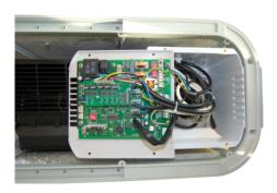
Fig. 20: Remove the control panel
