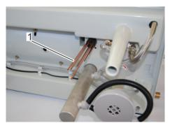
Fig. 41: Clean copper electrodes
