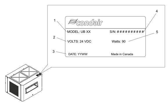
Figure 2 - Ultrasonic Blower Pack Specification Label
