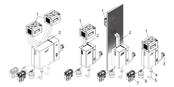
*Figure 5 - Ultrasonic Blower Pack Typical Installation with the Humidifier (Medium Humidifier Shown)*
