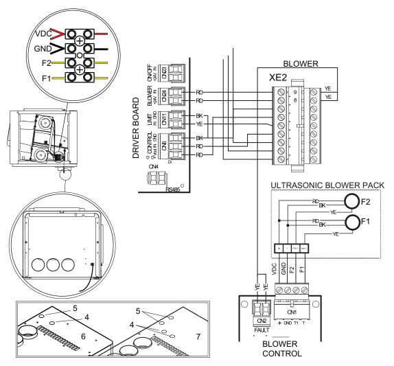
Figure 10 - Power and Security Loop Cables
