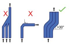
Figure 7 - Avoid horizontal sections and merging flexible tubes
