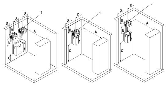
Figure 6 - Ultrasonic Blower Pack Clearance Suggestions
