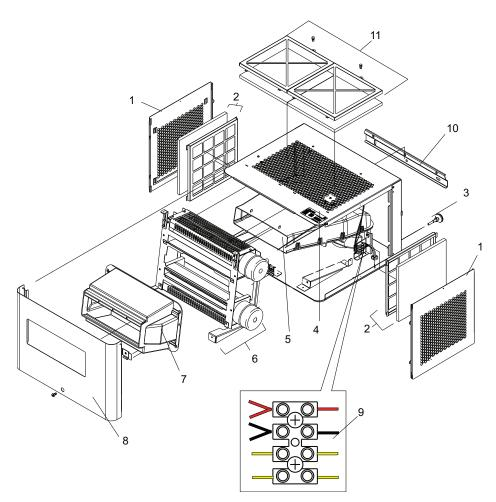
Figure 3 - Ultrasonic Blower Pack Components
