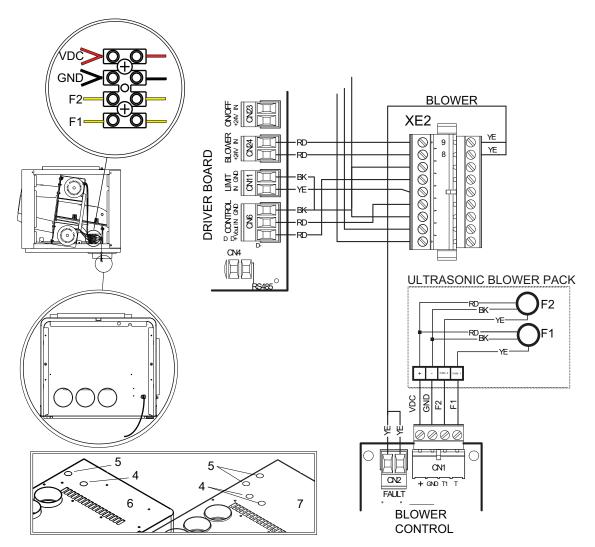
Figure 11 - Driver Board Connections
