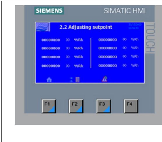
Force the HP pump to run by adjusting the set point in a section to 75%.
