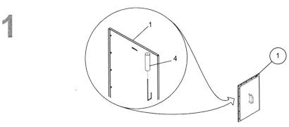
Ensure the sacrificial anode (4) is oriented upwards and rests over the bracket behind the tank door (1).
