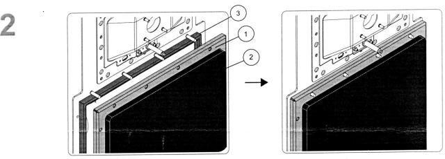
Place the gasket (3) and door (1) over the tank opening. Ensure the gasket is between the tank and the door.
