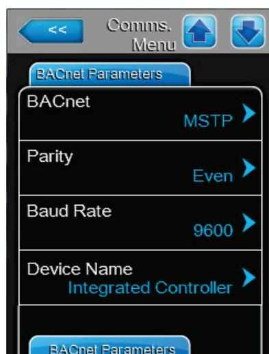
The following settings appear only if *BACnet* is set to "MSTP". **Note:** When set to BACnet MSTP the Nortec EL communicates as a BACnet slave only. BACnet master functionality requires installation of optional hardware.
