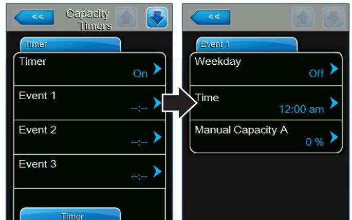
**Timer:** allows you to enable or disable the Manual Capacity timer function to reduce maximum output during selected days and times of the day.
