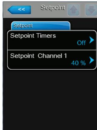
Allows you to set a fixed humidity setpoint without the use of timers.
