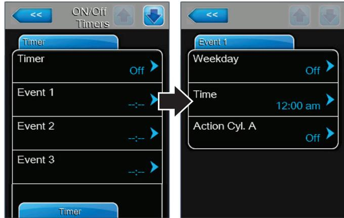
**Timer:** allows you to enable or disable the On/Off timer function.
