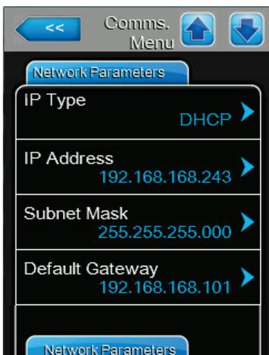
The following settings are used only for communications via the integrated BACnet IP protocol, Condair Online and web pages.
