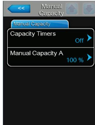
Allows you to set a fixed maximum output capacity without the use of timers.
