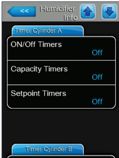
**Note:** The Timer Cylinder B tab appears only on units with dual steam cylinders that are set to work in independent mode. It is identical to the Timer Cylinder A tab.
