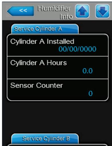
**Note:** The Service Cylinder B tab appears only on units with dual steam cylinders, and is identical to the Service Cylinder A tab.
