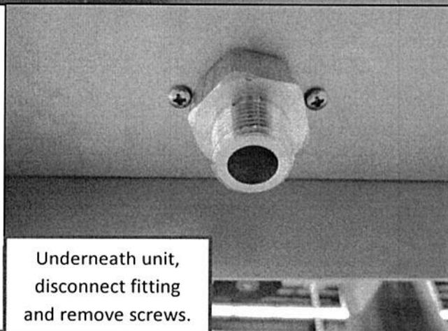
Underneath unit, disconnect fitting and remove screws.
